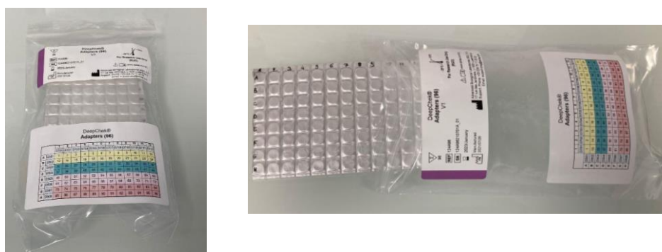
Figure 1: "Plate" format for a single and direct use for either 24, 48 or 96 samples
