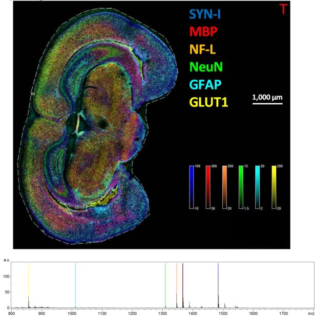
**Top:** Example Miralys<sup>™</sup> Results from Pre-Stained FFPE mouse brain tissue slide. MALDI mass spectrometry imaging was performed on a Bruker rapifleX<sup>™</sup> Tissuetyper with 20 µm spatial resolution. The image was generated from flexImaging with TIC normalization and the display intensity scale in absolute units.
