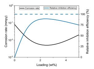
Corrosion performance of a structural steel coated with a 80 µm-thick acrylic waterborne dispersion as a function of the loading of B-LEAF h-BN relative to the dry coating. No other corrosion protective additives/pigments were used in the tests.
