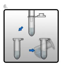
Gently remove the Eppendorf Tube from the end of the Compression Tube. It is appropriate to remove the Eppendorf Tube during expression if necessary due to foaming. Add preservative (not provided), if required, and close the lid on the tube tightly.
