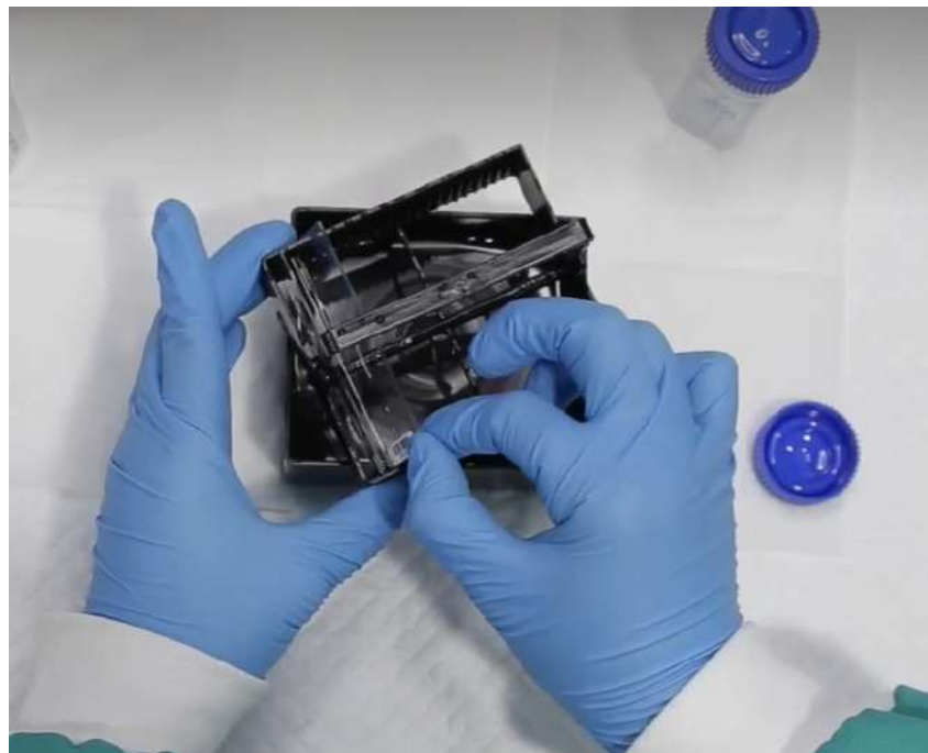
Figure 3. Slide staining dish and rack used in several wash and incubation steps throughout the assay procedure. The rack can hold up to 25 slides and has a lid (not part of the kit. BRAND™; Cat# BR471800-5EA).
