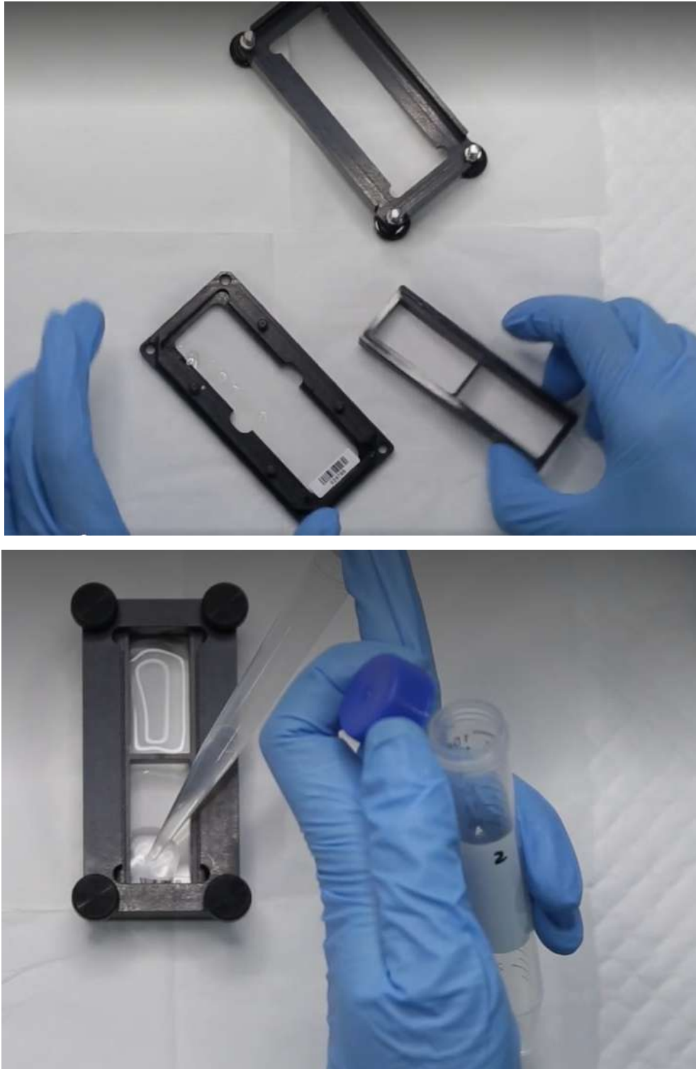
Figure 4. Prior to sample addition, the slide is inserted into the dual well chamber secured by a slide holder (upper panel). Once the slide is secured, the sample can be gently added (lower panel). Sengenics Dual-Well Chambers (Cat# 20010); Sengenics Slide Holders (Cat# 20020). These accessories are not part of the kit.
