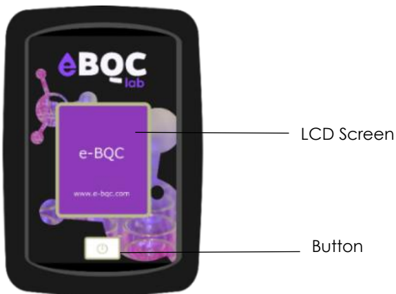
Figure 4. e-BQC lab Upper Panel
