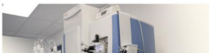
Q Exactive is a hybrid quadrupole-Orbitrap mass spectrometer
